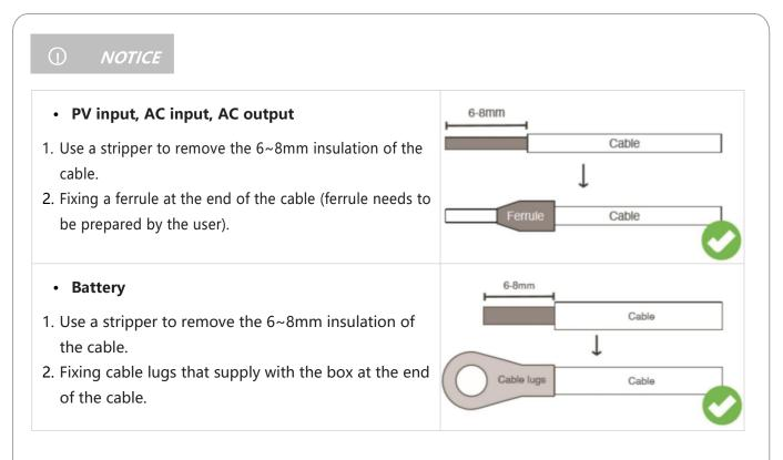
The wire diameter is for reference only. If the distance between the PV array and the inverter or between the inverter and the battery is long, using a thicker wire will reduce the voltage drop and improve the performance of the system.
